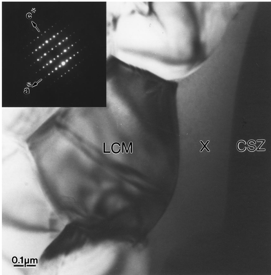
Figure 5 TEM image of \text{La}_{0.4}\text{Ca}_{0.6}\text{MnO}_3/\text{CSZ} diffusion couple fired for 15 min at 1350^\circ\text{C} . Formation of a secondary phase (marked by X), \text{Ca}_6\text{Zr}_{19}\text{O}_{44} , at the interface is shown. (inset) [010] zone-axis pattern of \text{Ca}_6\text{Zr}_{19}\text{O}_{44} . The a^* - and c^* -directions of the hexagonal cell are indicated. The crystal structure indexing is based on the hexagonal cell with a_H = 27.366 \text{ \AA} and c_H = 11.713 \text{ \AA} given by Yin and Argent [20].
